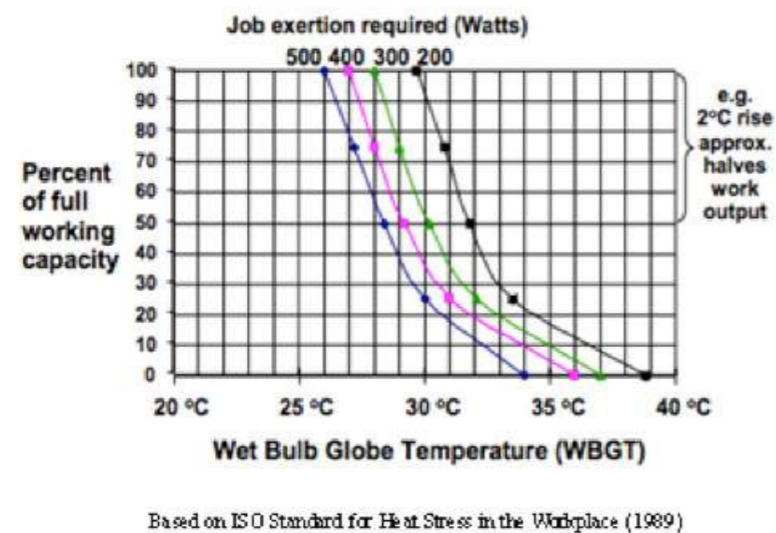
Figure 1: The relationship between heat and work - a function of ideal human physiology and a pointer to fundamental temperature thresholds. 9
